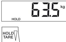
**0.0** appears in the display if the scale has no load on it, otherwise the current weight.
