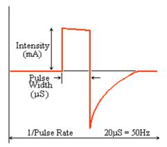
As can be seen from the diagram above of a single stimulation pulse the stim is balanced thus there is no DC component. This means that during stimulation session there is no residual build up of energy at the electrode site.
