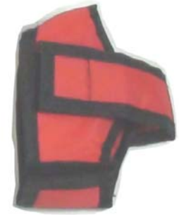
Hinge wrap for front fork
