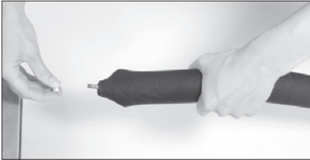
1. Remove nylon locknut [32] from spring bolt [31].
