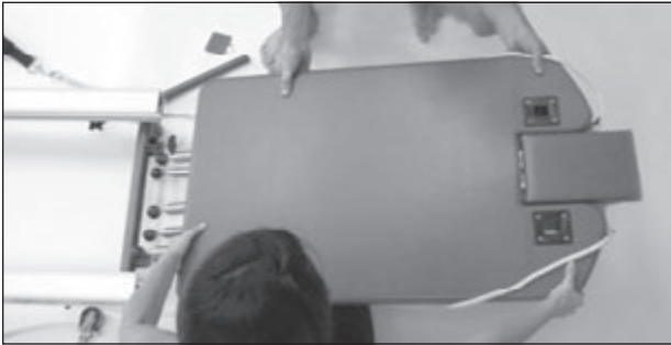
4. Align fixed rollers [37] with c-channels [51], then adjust floating rollers [38] as necessary before guiding carriage [15] into rails [14].
