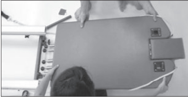
1. Remove the carriage [15] and place face down on a blanket or soft surface. See page 23 for full instructions.
