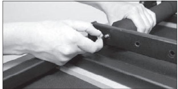
4. Thread nylon locknut [32] onto spring bolt [31].
