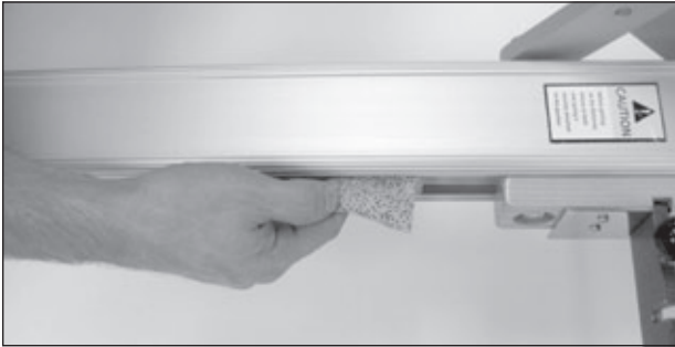
2. Wipe inside of aluminum rails (c-channels) [51] with a damp cloth using water only to remove dust or dirt. Spray onto cloth first. Avoid spraying liquid directly onto surfaces, rollers or rails. Insert carriage stopper [47] in one of six positions.
