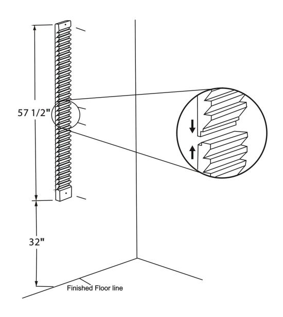
Note: Recommended mounting height is approximately 32"from finished floor.
