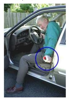
Insert the Handybar® into the U-shaped striker plate located on the driver and passenger-side door frames of the vehicle.
