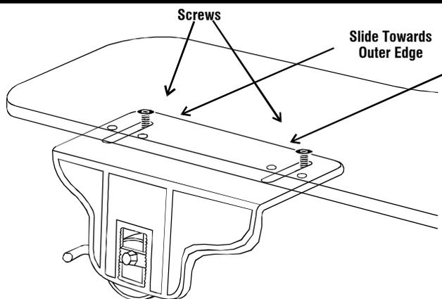
1. Loosen the screws that hold the E-Z Lock Clamps to the tray. This allows the clamps to be adjusted to the **WIDTH** of the armrests.
