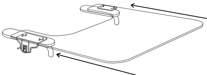
5. Center the tray on the chair. Adjust the clamp assemblies so the edge of each clamp fits against the side of the armrest. The round **Cam** should be below the armrest for now. Tighten the screws that hold the clamps to the tray. The screws should be tightened so the tops are flush with the surface of the tray.
