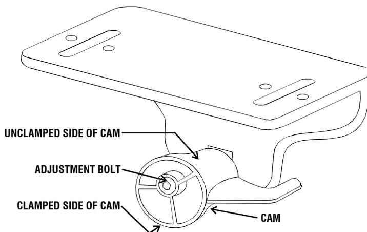
6. With the **UNCLAMPED** side of **Cam** facing the underside of the armrest, push **Cam** up in **Adjustment Notch** slide until the **Cam** loosely contacts underside of armrest. Push in **Adjustment Nut** and hold it in place within the notches. Rotate **Cam** so the **CLAMPED** side tightens up against the underside of the armrest. Test-fit the **Cam** up and down in different positions, to determine best position.
