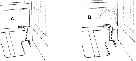
To remove drop-seat, slide seat back so that J-Hooks are not engaged by hold-down brackets, or loosen the wing nuts and slide the hold-down bracket away from the J-hook. Lift seat up and off wheelchair seat rails.
