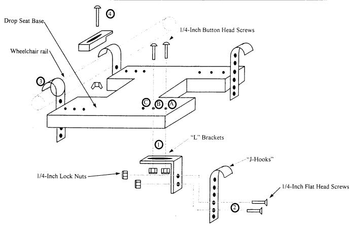
**Step 1.** Mount each L-Bracket beneath drop-seat using two ¼-inch button-head screws and two lock nuts. For 18-inch wheelchairs, use screw holes A and B. For 16-inch wheelchairs, use screw holes B and C. (See illustration above). Note that the drop-seat must rest on the *slotted* side of the L-bracket. Hand tighten only. Some final width adjustment may be required.
