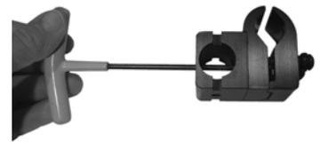
2. Loosen Clamp Screws using large T-Wrench **Do not remove screws** and open clamp to its widest position by pushing the Moveable Jaw forward and pulling it outward as shown in photo.
