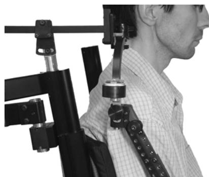
**Note:** *Positioning of the Shoulder Link may require loosening of the two screws on the Shaft Mount Base or repositioning the Mount Links*
