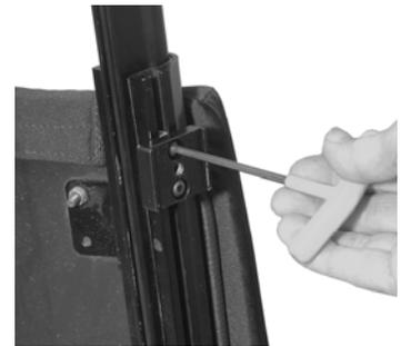
3. Orient the Arm Mount Base as shown in illustration. Insert the Mount Base Screw (supplied with Arm Mount Base) thru the Attachment Hole to the MR-8 Mount Adapter. Using the large T-Wrench secure these two parts.
