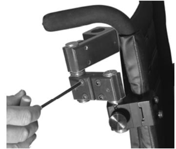
8. Hold the Pitch Mount Shaft so that the black Pitch Pivot is at the proximal end, the hole through the Pitch Pivot is in the line of progression of the chair and the plate of the pivot is facing laterally. Insert the Pitch Mount Shaft into the Shaft Mount Base. Snug but do not tighten the Shaft Screws on the Shaft Mount Base.
