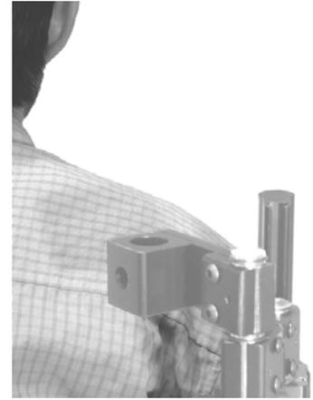
7. Snug but do not tighten the **six** Clamp Screws using the Large T-Wrench. *Add enough tension so that the joints do not move easily but can be repositioned if required to optimize the arm alignment.*
