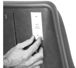
4. Use drill bit supplied and drill the two marked holes.
