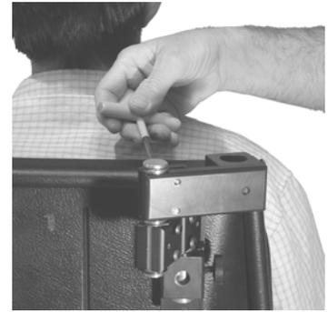
10. Snug but do not tighten the **six** Clamp Screws using the Large T-Wrench. *Add enough tension so that the joints do not move easily but can be repositioned if required to optimize the arm alignment.*
