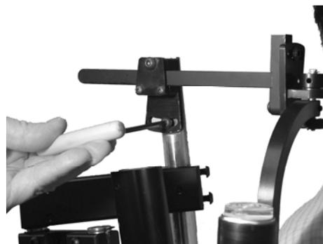
2. With the aid of the Bubble Level position the Pitch Link so that it is horizontal and parallel to the floor.
