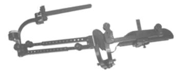
3. Using the medium T-Wrench remove the **Four** screws that connect the sections of the upper and lower Humeral Elevating Links
