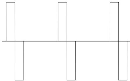
Figure 9.12 – TENS Waveform
