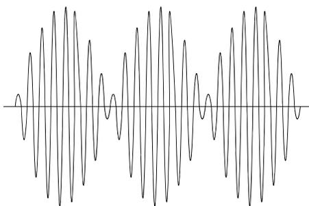
Figure 9.8—2-Pole Interferential Waveform
