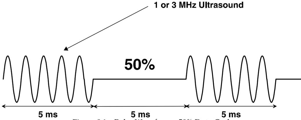
Figure 9.1 – Pulse Waveform – 50% Duty Cycle
